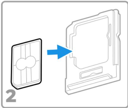
**Note:** Always power off the computer before attempting to install or remove a nano-SIM card.
