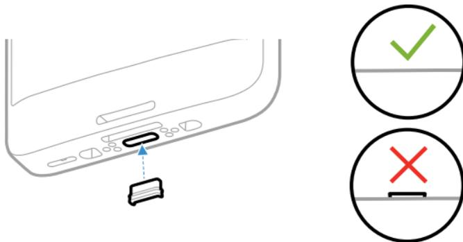
**Note:** *Verify the plug is properly installed if intermittent charging and/or communication issues occur when the computer is placed in an accessory.*
