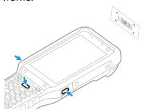
4. Release the Scan button when the computer beeps, and the Scan Status LED briefly turns on. The barcode information is entered into the application in use.
