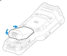
2. Press down on the battery until the battery latch clicks.
