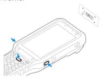
7. Release the Scan button when the computer beeps, and the Scan Status LED briefly turns on. barcode information appears on the screen.
